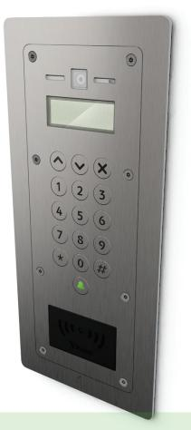
The Net2 Entry panel is a robust door entry panel incorporating both door entry and access control functions. It is powered using power over Ethernet (PoE) and communicates with the other elements of the system using IPv6, providing 'plug and play' installation. Each panel is associated with a Net2 Entry control unit which is the interface to the door hardware.
